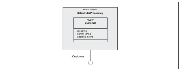
Figure 8: Interface specification data model for interface ICustomer
