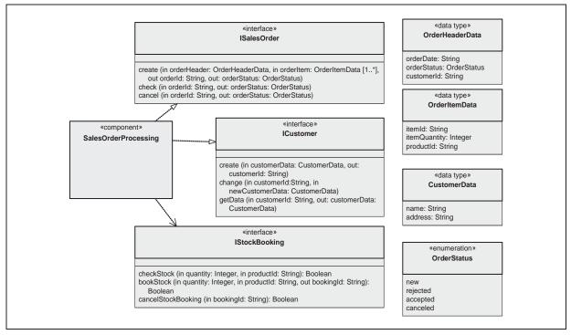
Figure 2: Interface specification for component SalesOrderProcessing
