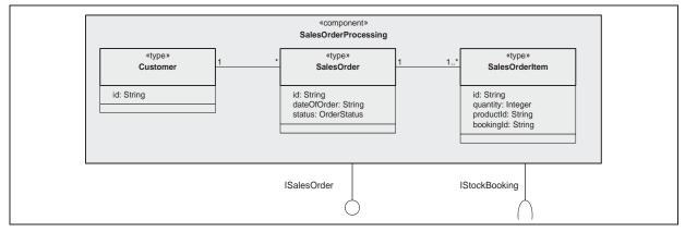
Figure 9: Interface specification data model for interface ISalesOrder
