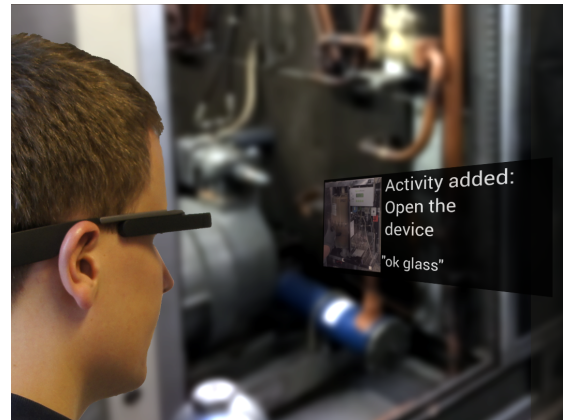
Fig. 7: Smart glasses-based modelling system
