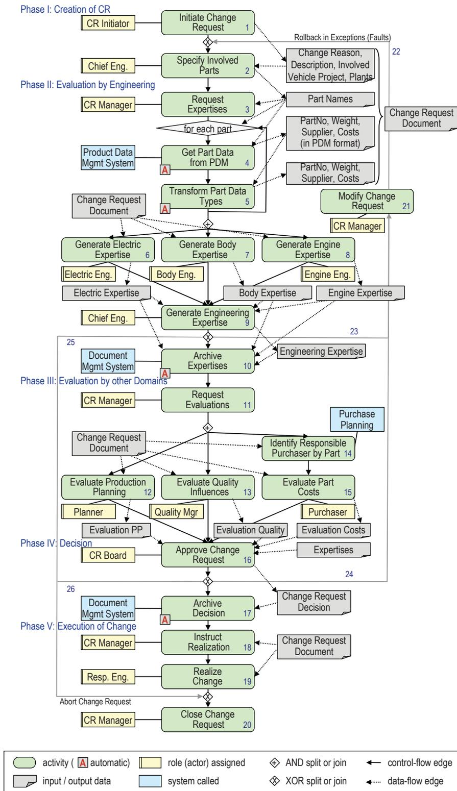
Figure 4: Process Model of a Change Request (CR)
