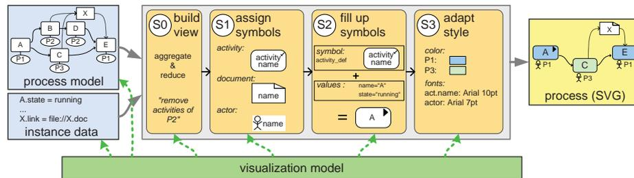
Figure 6: Generating a Process Visualisation in Proviado
