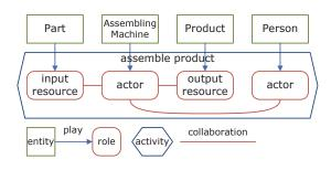
Figure 3: Role-based specification of the activity assemble product
