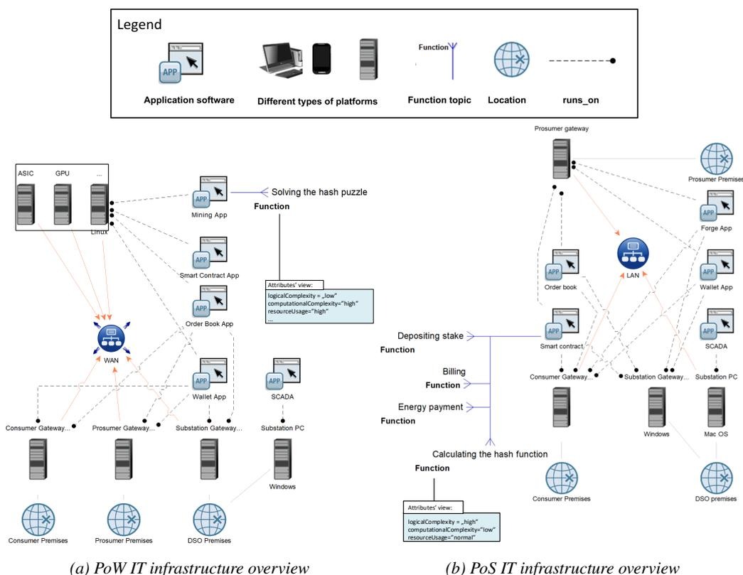
Figure 4: IT Infrastructures of Alternative Consensus Mechanisms, modeled using extended ITML
