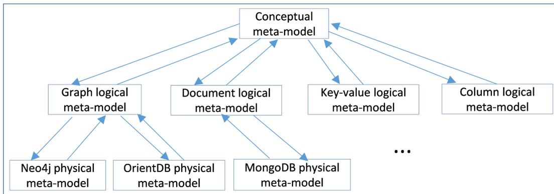
Figure 3: Recommended paths for NoSQL database roundtrip engineering
